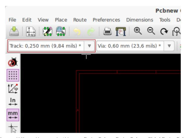
16. If you would like to add more track widths go to: **Design Rules** → **Design Rules** → **Global Design Rules** tab and at the bottom right of this window add any other width you would like to have available. You can then choose the widths of the track from the drop-down menu while you lay out your board. See the example below (inches).
